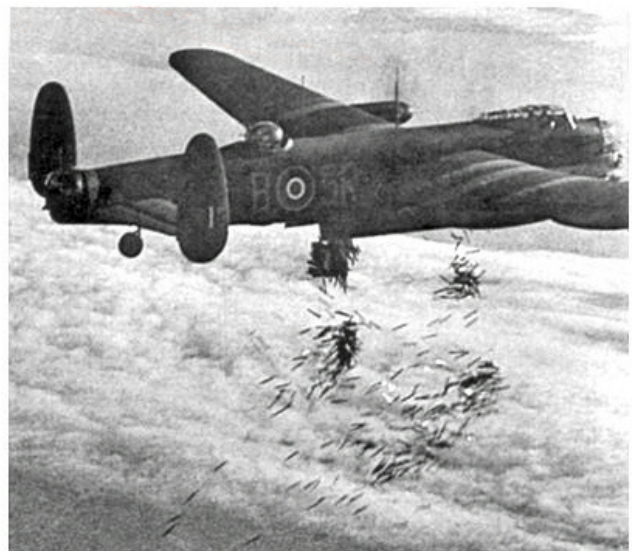
"Window" (left) and incendiary and Blockbuster bombs (right) dropped from Avro Lancaster over Duisburg in 1944
